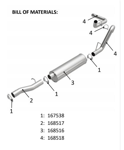
(Carefully read all instructions before installation) Disconnect the vehicle's battery before removal of the OEM exhaust system. This will prevent electrical accidents and will reset the computer if it applies to the vehicle. Remove existing exhaust system from the vehicle. Only remove parts that will be replaced. Clean existing flange with a wire brush to ensure proper sealing.
